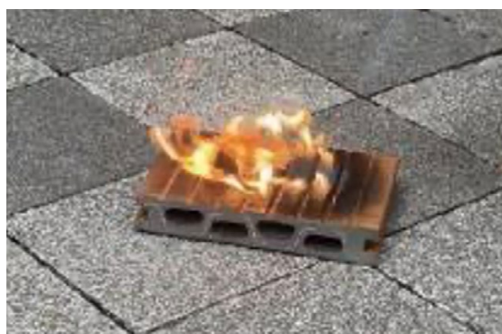
↓ 阻燃、遇火自熄 flame retardant and self-extinguishing ↓
