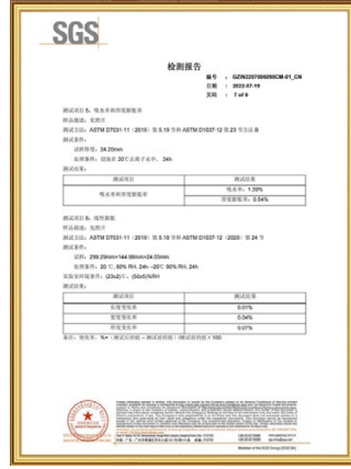
吸水率和厚度膨脹率 Water Absorption and Thickness Expansion
